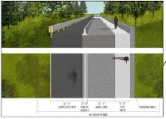
**Side Path** - west side of Sandy Avenue Option B - replace rehide travel lane with a 12' wide shared use path separated from the vehicles by permanent barrier. Sandy Are widened to accommodate new shared use path.
