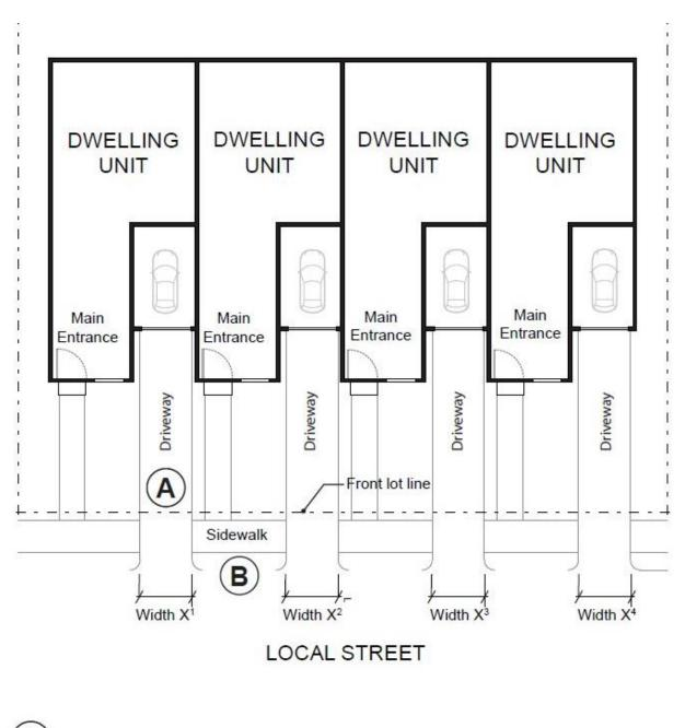
A) X<sup>1</sup> + X<sup>2</sup> + X<sup>3</sup> + X<sup>4</sup> must not exceed 32 feet per frontage,
